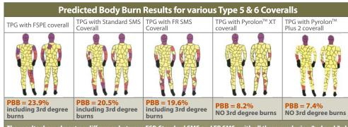
The results show almost no difference between FSP, Standard SMS and FR SMS, with all three producing 2nd and 3rd degree burns. Pyrolon™ Plus 2 and XT coveralls produce much lower predicted burns and no 3rd degree burns
